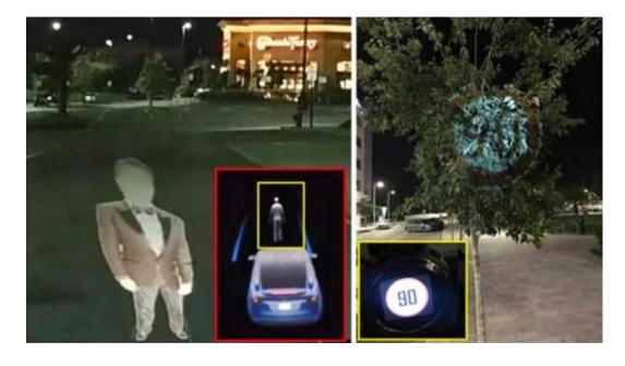
Figure 1.6 Tesla's autopilot fooled by phantom images
